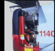
**Full opening rear engine compartment** allows daily machine servicing to be conveniently accomplished from ground level.
