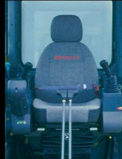
**Multi-adjustable suspension seat** provides for long days of productive operation with minimal operator fatigue.
