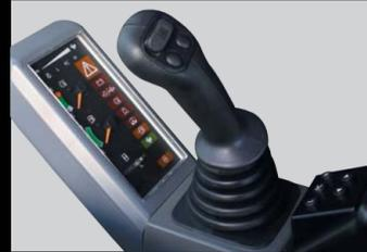
**One touch engine decelerator** installed on the right hand joystick reduces fuel consumption when the excavator is temporarily idled.
