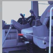
**Console safety lockout levers** disable travel and operating controls for safe entry and exit from the excavator.
