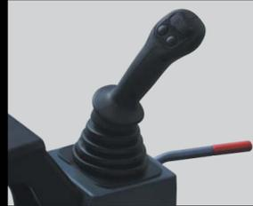
**Hydraulic attachments** are operated by momentary push button or proportionally controlled by the slider switch on the joystick.
