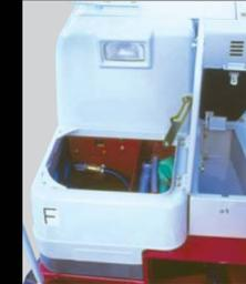
**The fuel system automatically bleeds air** from fuel lines on a fuel-depleted machine saving on time, tools and unnecessary service calls.
